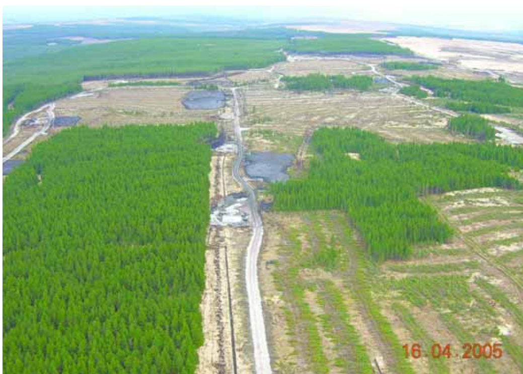
Figure 10 : Derrybrien, Co. Galway. Tracks, turbine bases on the left of the main track, ditches, cable trenches, dumped peat and clear felling, all contribute to peat damage and CO 2 release.
