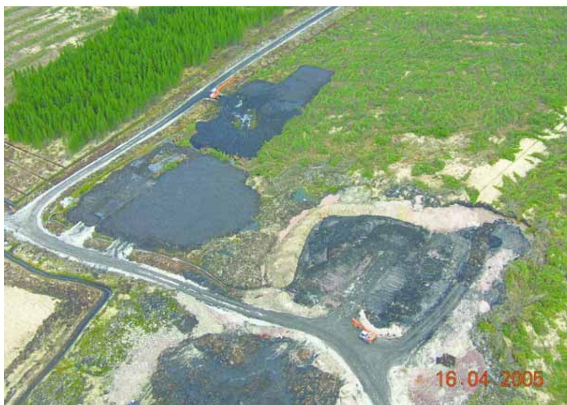
Figure 6: Damaged bog surrounding a turbine base at Derrybrien wind farm (Irish Republic). Also shown are dumps of peat left to oxidise, tracks and drainage ditches.
